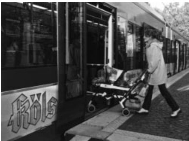
Level access from platform to vehicle in Germany.
